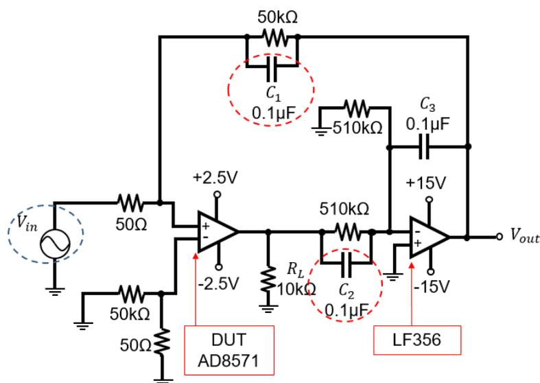
Fig. 4. Frequency characteristics measurement circuit
