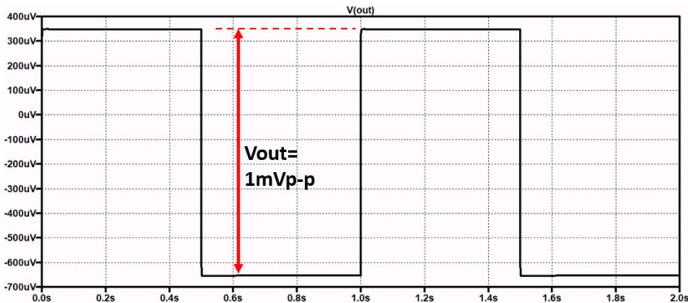
Fig. 7. Offset voltage measurement result
