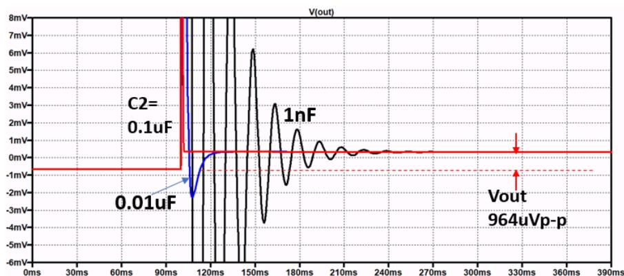
Fig. 12. PSRR simulation result when  $C_2$  is varied.
