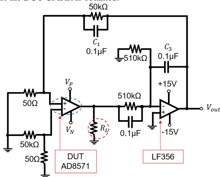
Fig. 10. CMRR measurement circuit
