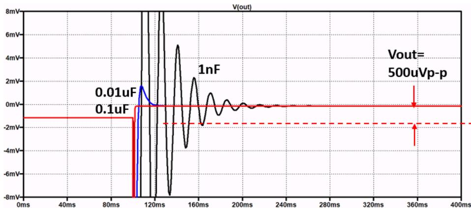
Fig. 11. CMRR simulation result when  $C_2$  is varied.
