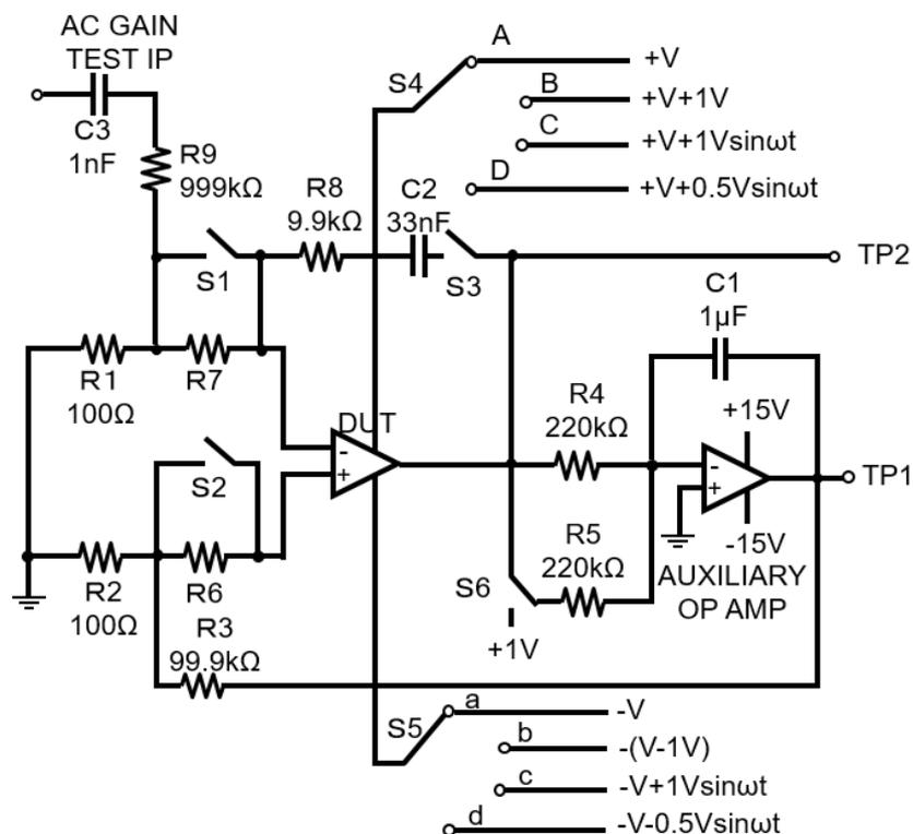
Fig. 1. Operational amplifier measurement circuit using the NULL method.
