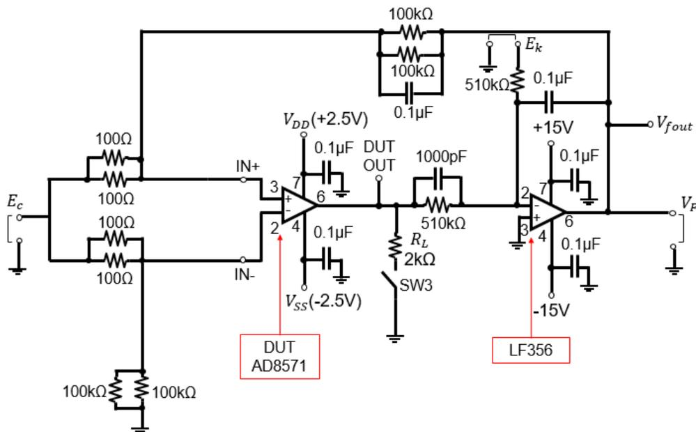
Fig. 2. Experimental circuit using the NULL method
