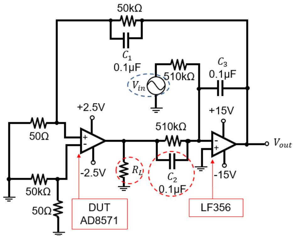
Fig. 8. Open loop gain measurement circuit
