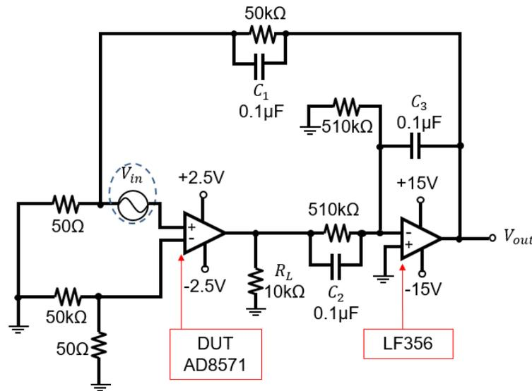
Fig. 6. Offset voltage measurement circuit
