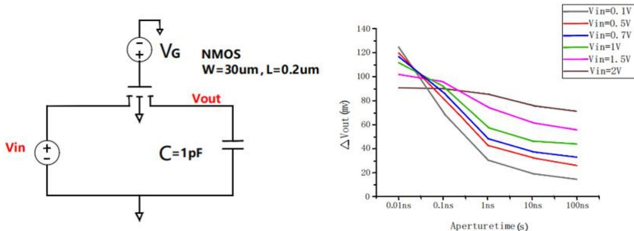
Fig. 8 Pedestal error in NMOS switch sampling circuit for various aperture time.
