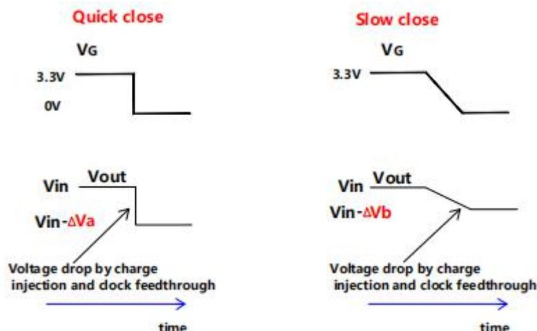
Fig. 7 Charge injection in sampling circuit for quick and slow turn off.
