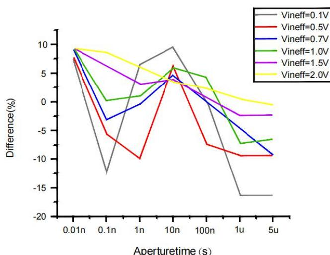
Fig. 10 Difference of pedestal errors between NMOS and PMOS switch sampling circuits.  $V_{ineff}$  is defined as  $V_{in}$  for NMOS switch sampling circuit, while  $V_{dd}-V_{in}$  for PMOS one.
