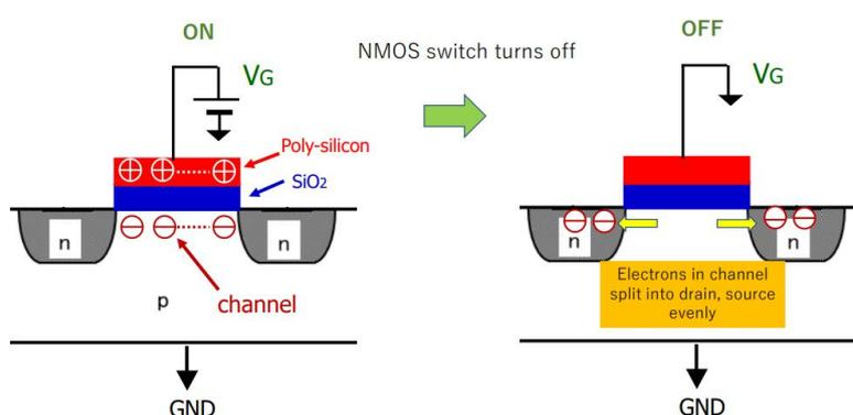
Fig. 6 Channel charge of NMOS. (a) ON state. (b) Turn off transition.
