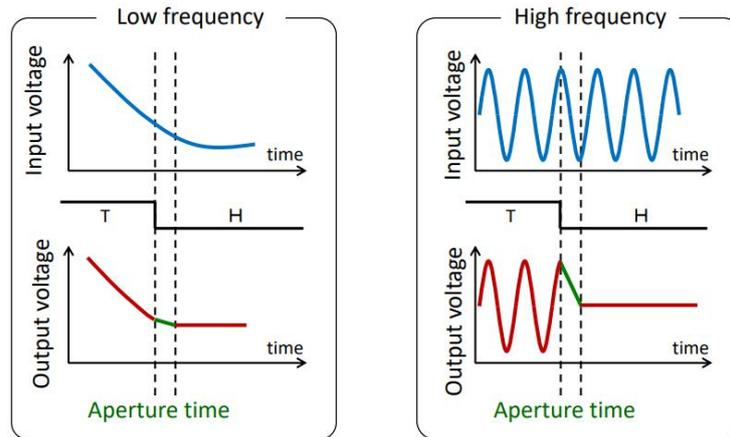
Fig. 3 Finite aperture time effects for low signal and high frequency signal sampling.
