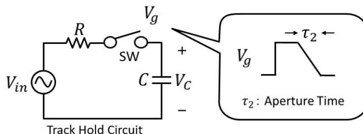
Fig. 5 Sampling circuit model with finite aperture time  $\tau_2$  and switch on-resistance  $R$ .
