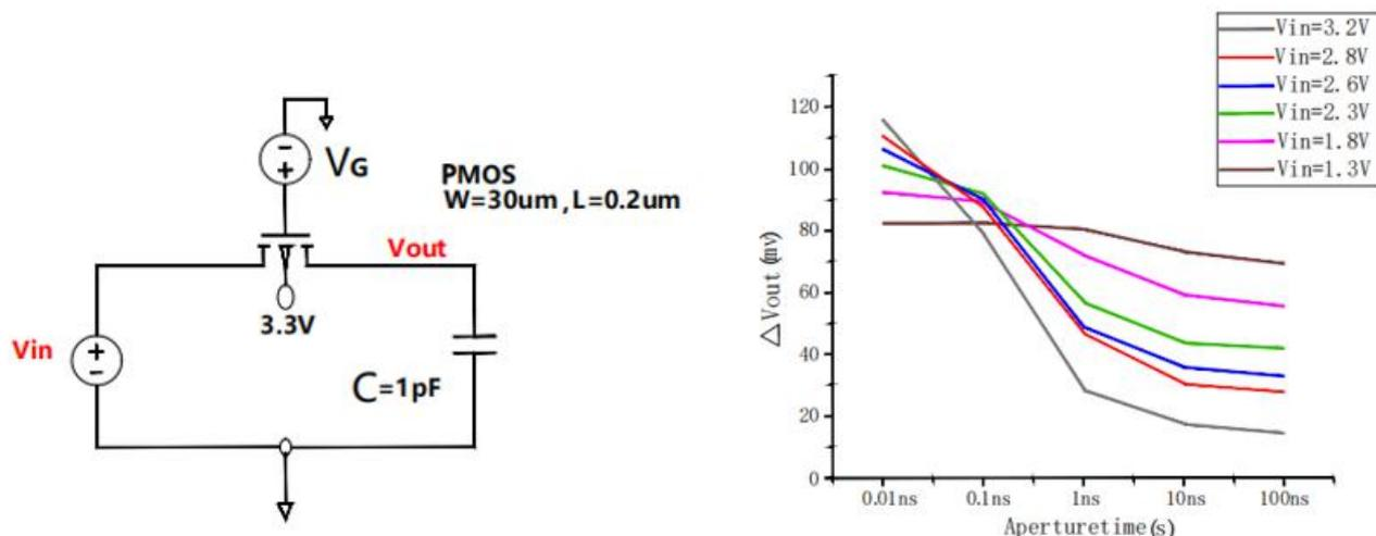
Fig. 9 Pedestal error in PMOS switch sampling circuit for various aperture time.
