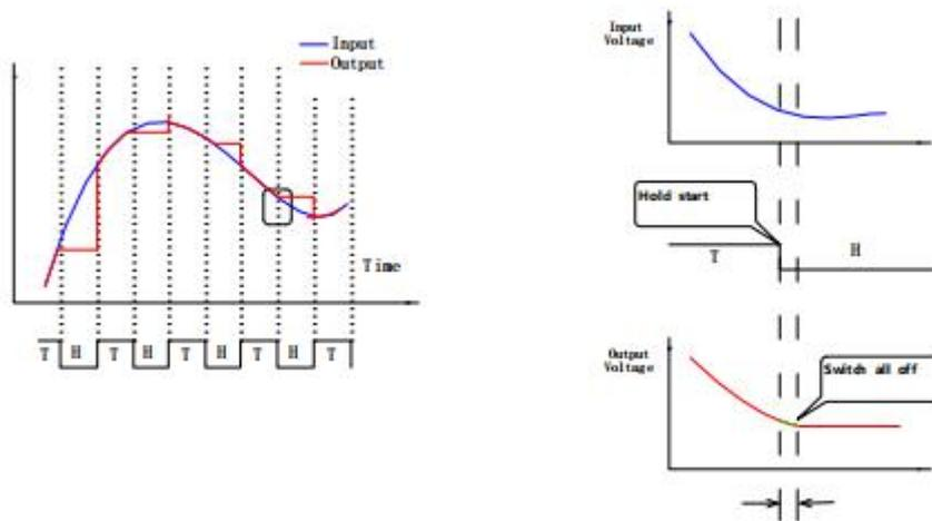
Fig. 2 Definition of aperture time in a sampling circuit.
