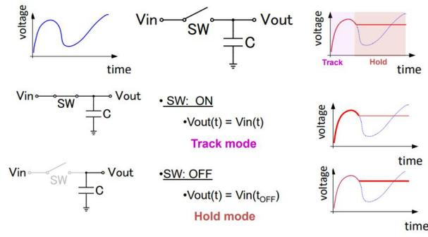
Fig. 1 Waveform sampling and sampling circuit.
