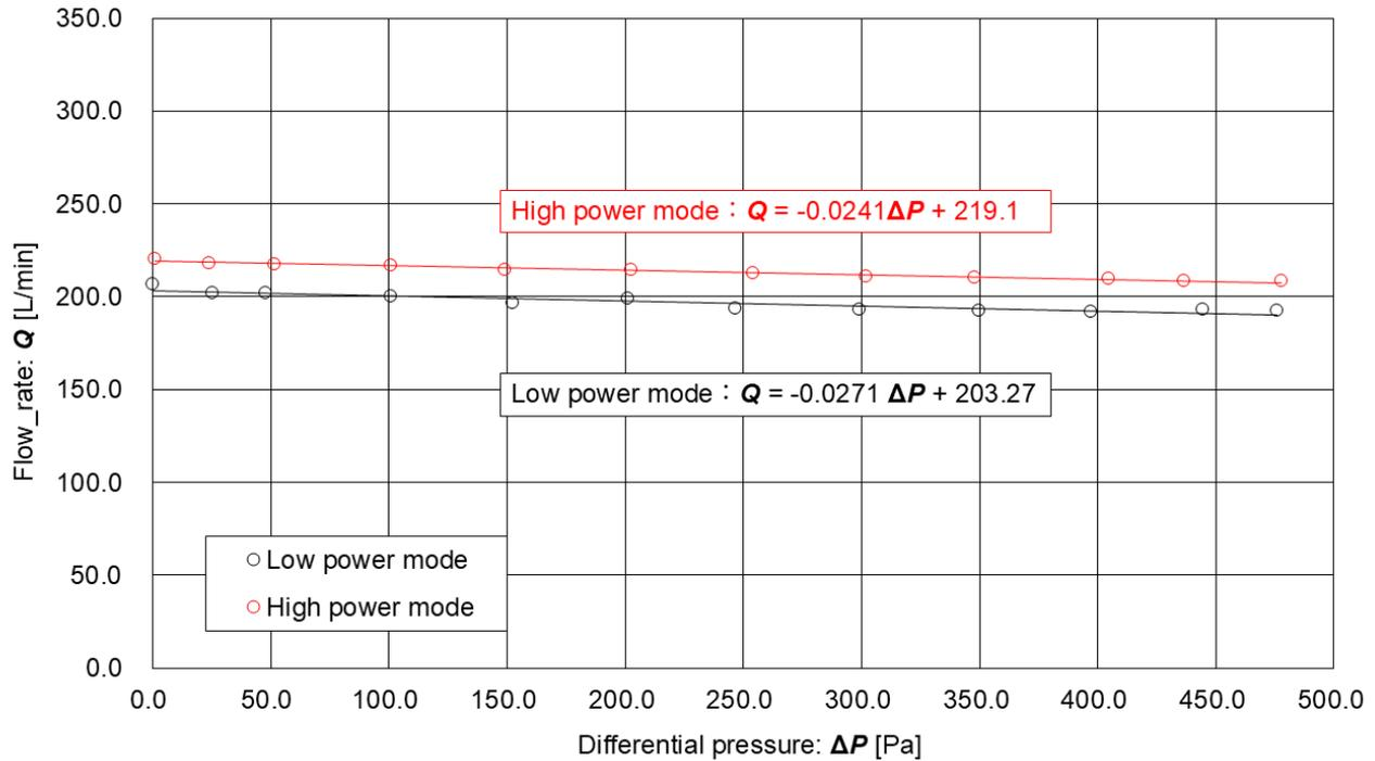
Fig. 6. Result of the relationship between differential pressure and flow rate for 3M
