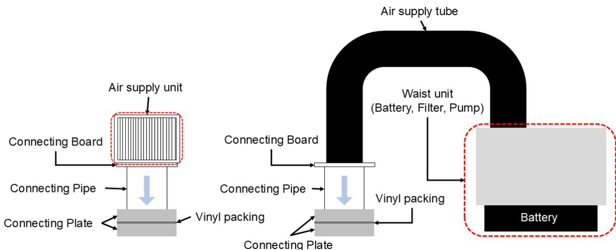
(a) Air supply unit with connecting attachment
