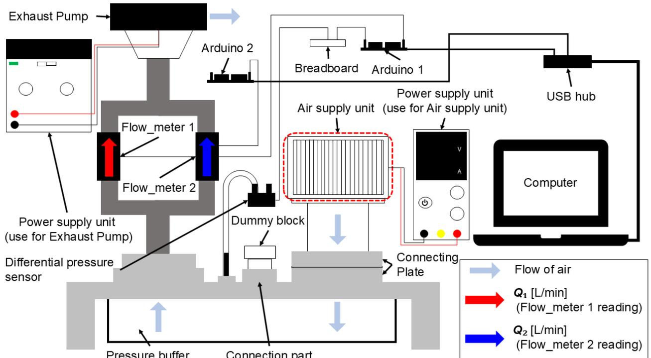
Fig. 1. A schematic diagram of "The evaluation device for differential pressure dependence of flow rates".
