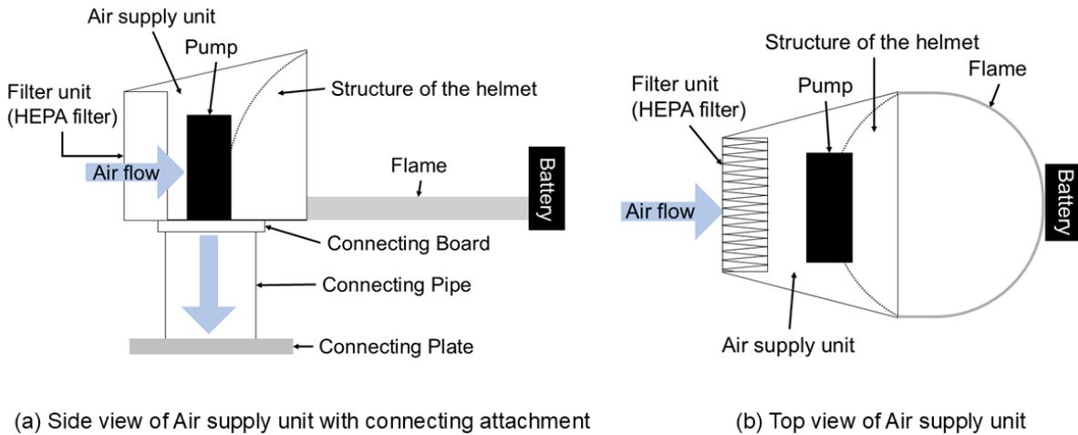
**Fig. 3. Side view and Top view of Air supply unit**
