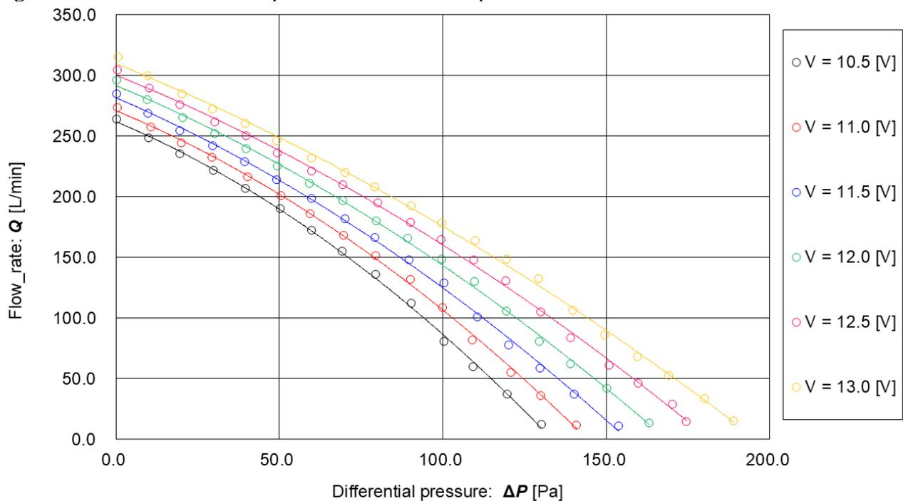
Fig. 5. Result of the relationship between differential pressure and flow rate for Air supply unit
