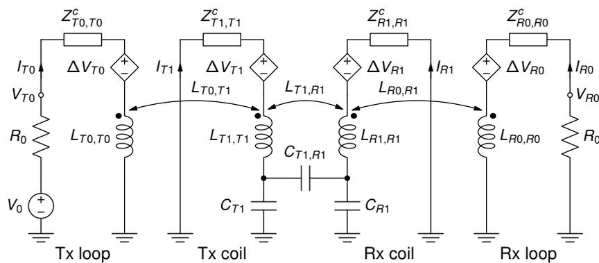
Fig. 4. Equivalent circuit of the WPT system.
